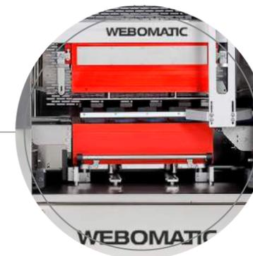
**Die lifting device** with a reliable knee lever system that is guided by a precise 4-column design and completely service-free.
