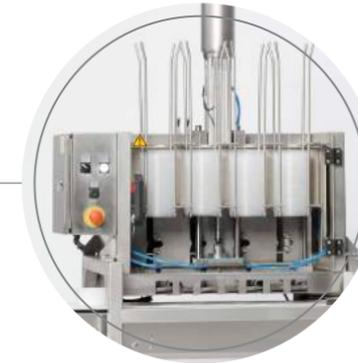
**Use a tray denester** in front of infeed-conveyor for automatic denesting of trays.
