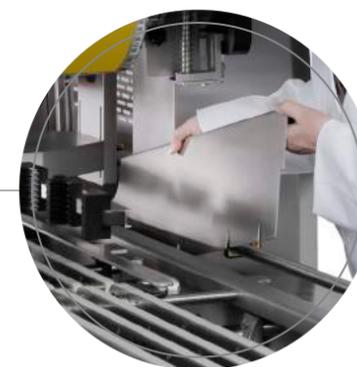
With the **positioning template**, a quick and time-efficient tray fitting is ensured for every die set.
