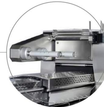
**Duplex top film unwinding** for faster top film changes and less downtime during the packaging process.
