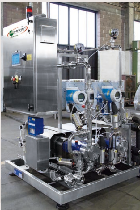
Counter-liter Mixing system with flowmeter
